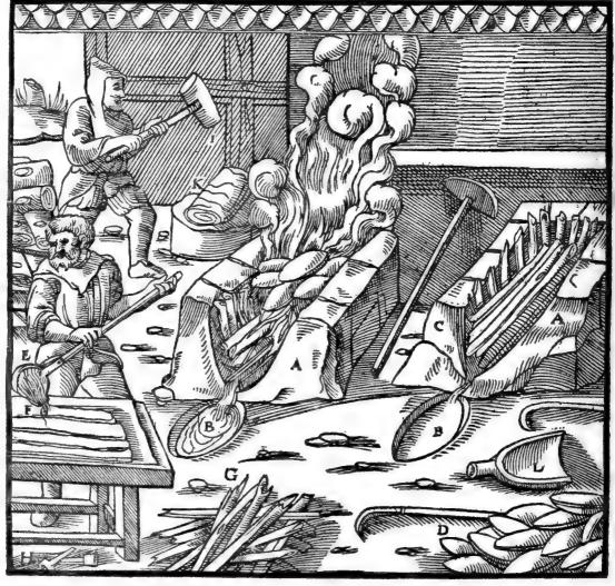
A—HEARTHS. B—DIPPING-POTS, C—WOOD, D—CAKES, E—LADLE, F—COPPER PLATE, G—LATTICE-SHAPED BARS, H—IRON DIES, I—WOODEN MALLET, K—MASS OF TIN BARS, L—SHOVEL,
